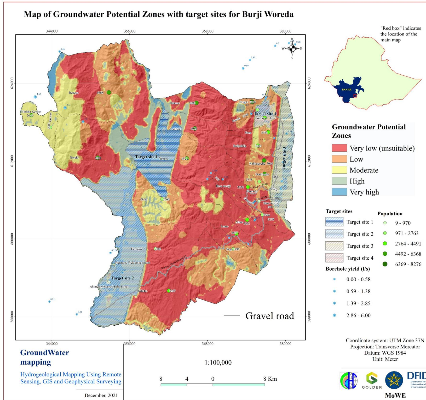
Figure 5.48. Map of groundwater potential zones with selected target sites in Burji Woreda
