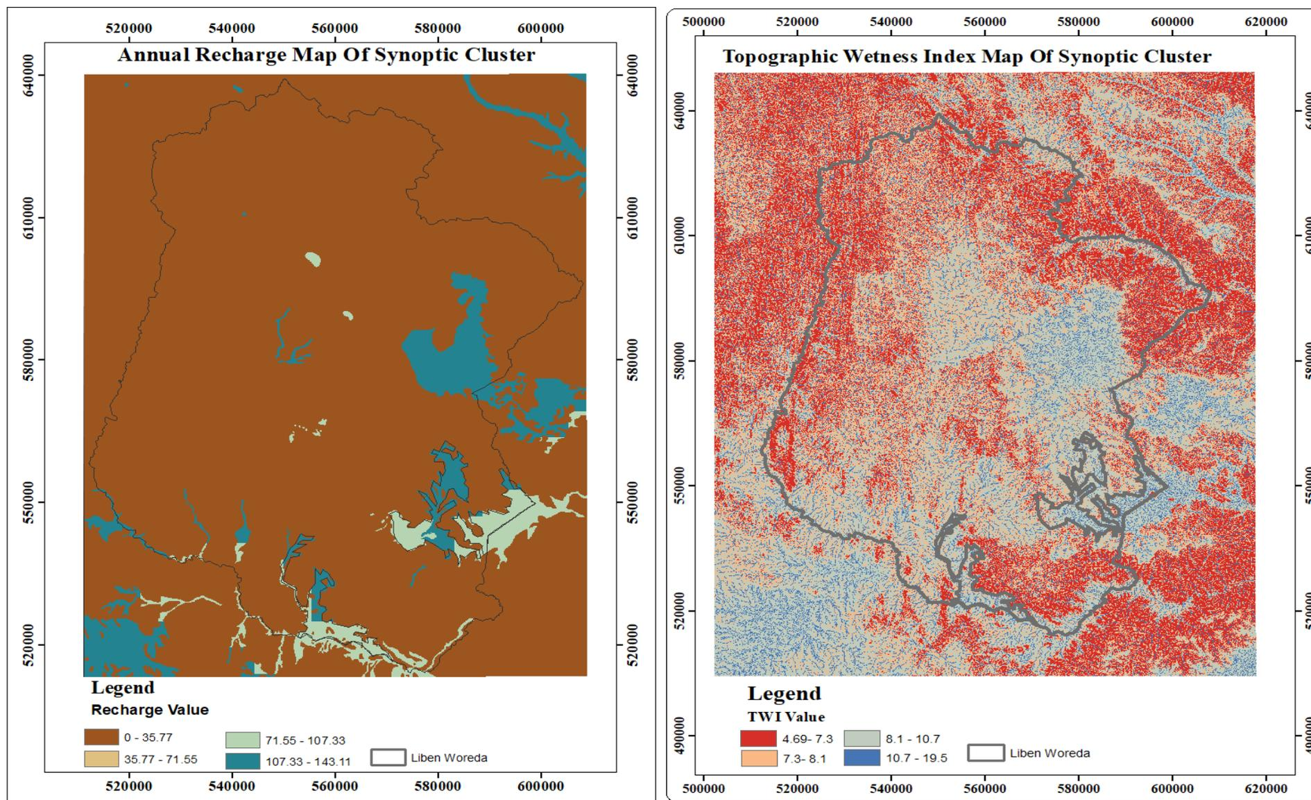
Figure 4.25. Map of TWI (right) and annually recharge (left) for Liben Woreda in synoptic view
