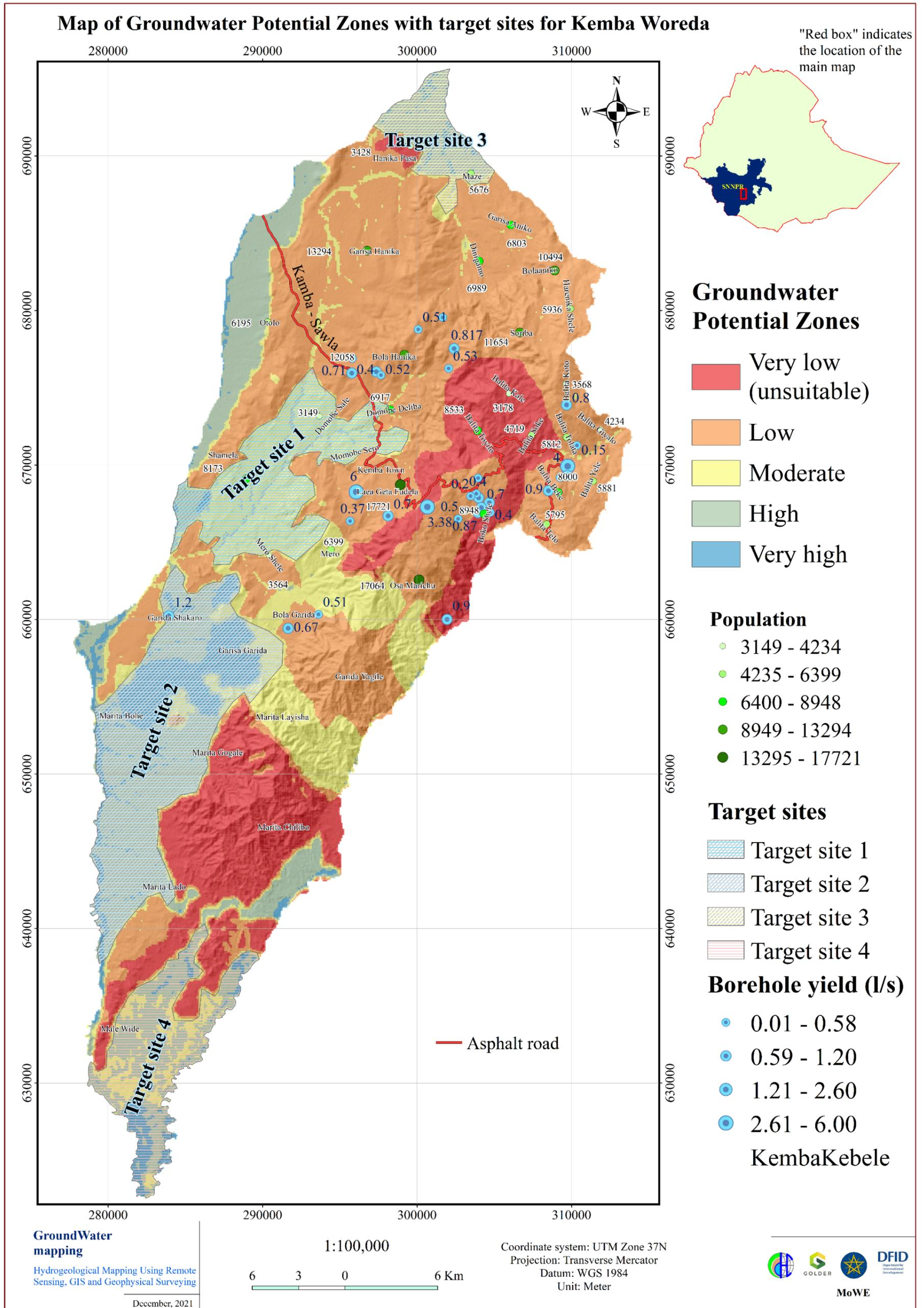
Figure 5.40. Map of groundwater potential zones with selected target sites in Kemba Woreda
