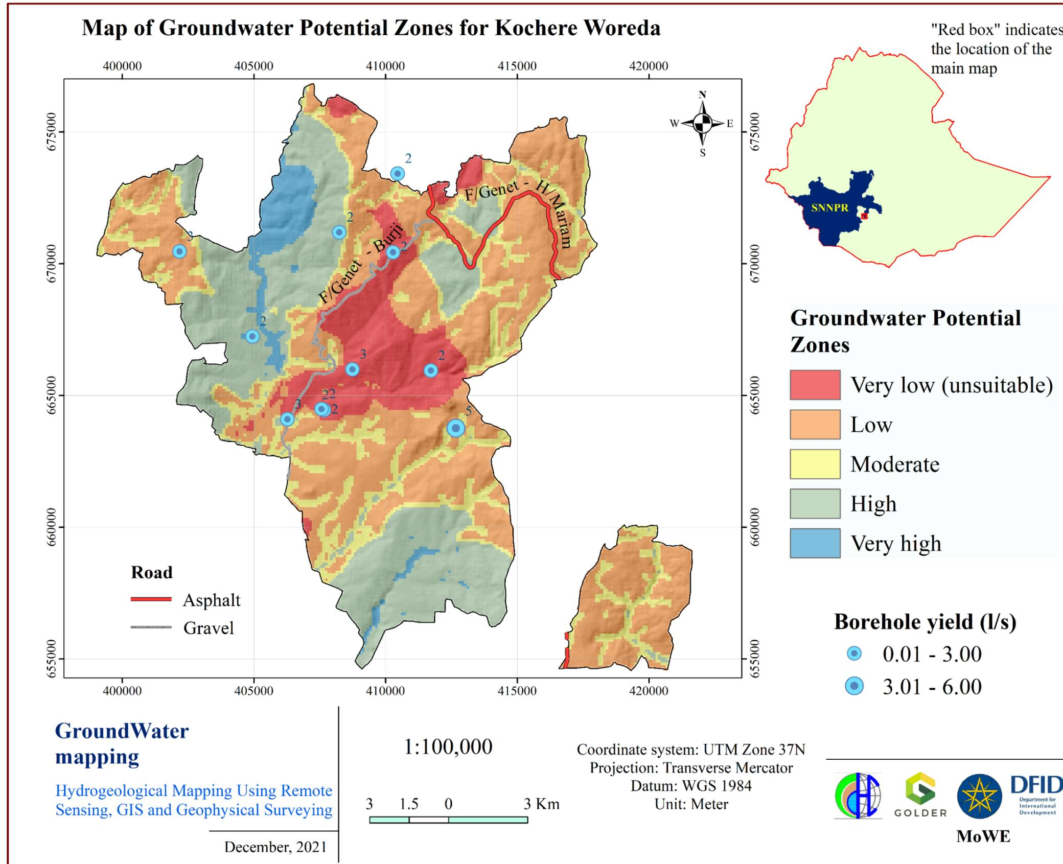
Figure 5.29:- Map of groundwater potential zones showing five zones identified by the GIS overlay analysis in Kochere Woreda
