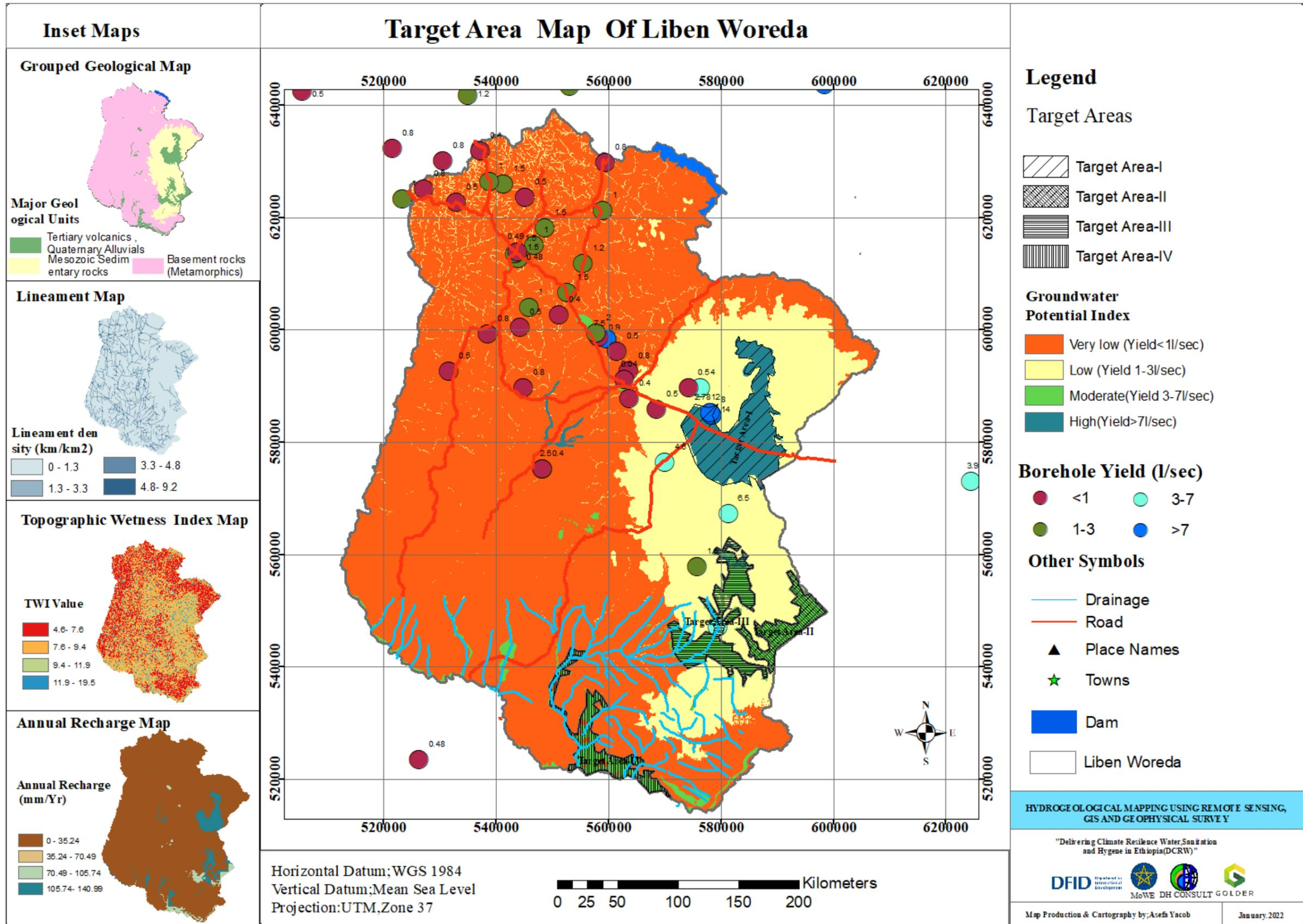
Figure 5.112: Map of groundwater potential zones with selected target sites in Liben Woreda
