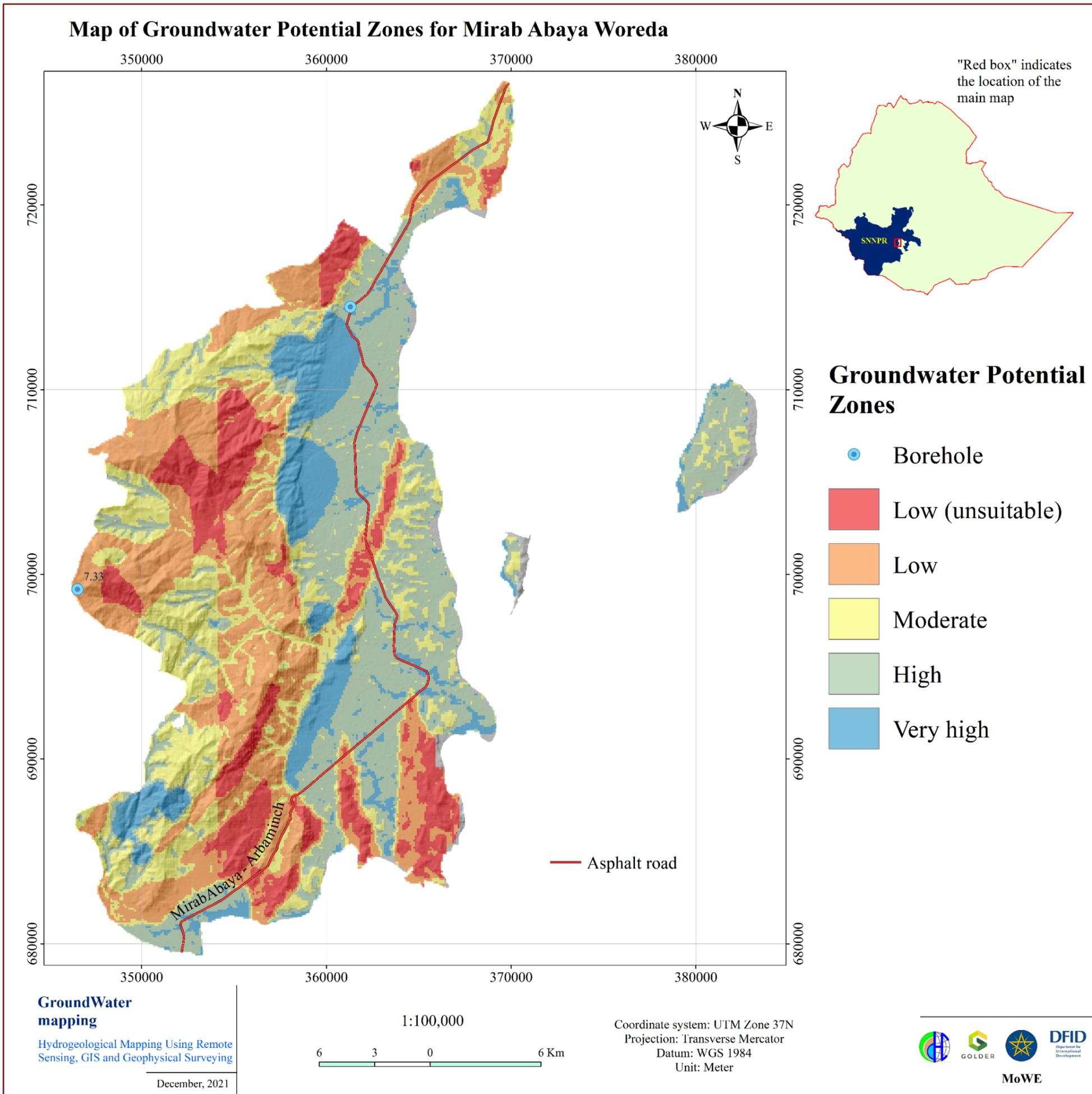
Figure 5.13. Map of groundwater potential zones showing five zones identified by the GIS overlay analysis in Mirab Abaya Woreda
