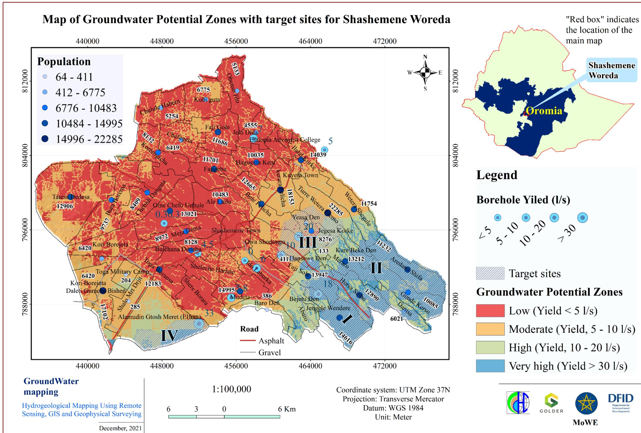
Figure 5.102: Map of groundwater potential zones with selected target sites in Shashemene Woreda
