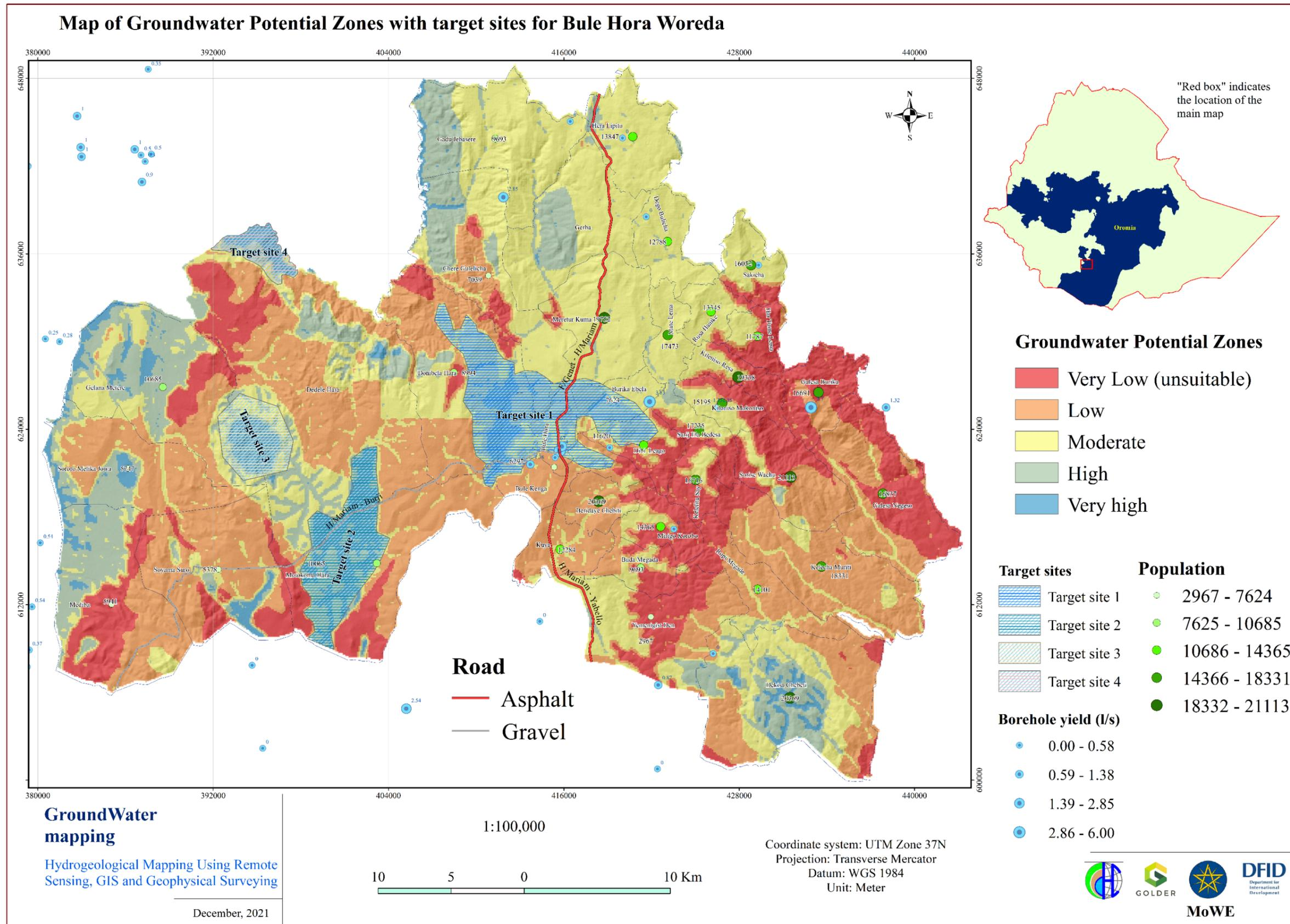
Figure 5.8. Map of groundwater potential zones with selected target sites for Bule Hora Woreda
