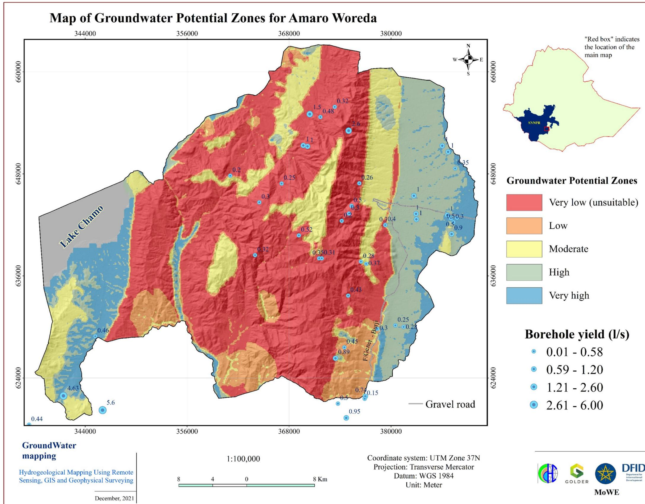
Figure 5.53. Map of groundwater potential zones showing five zones identified by the GIS overlay analysis in Amaro Woreda
