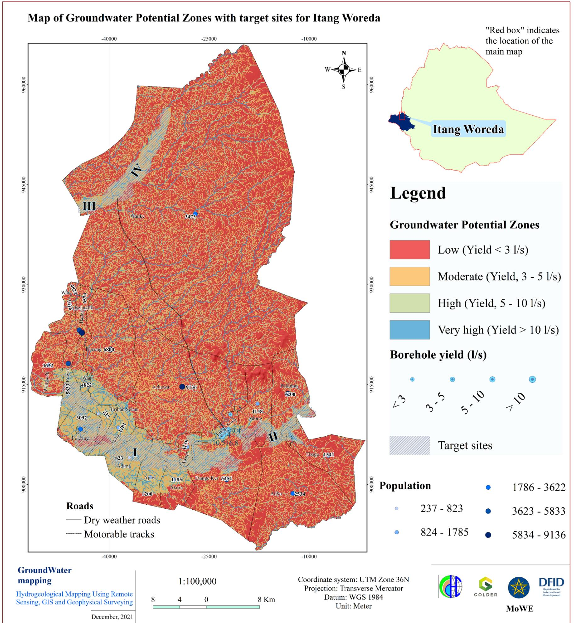
Figure 5.90: Map of groundwater potential zones with selected target sites in Itang Woreda
