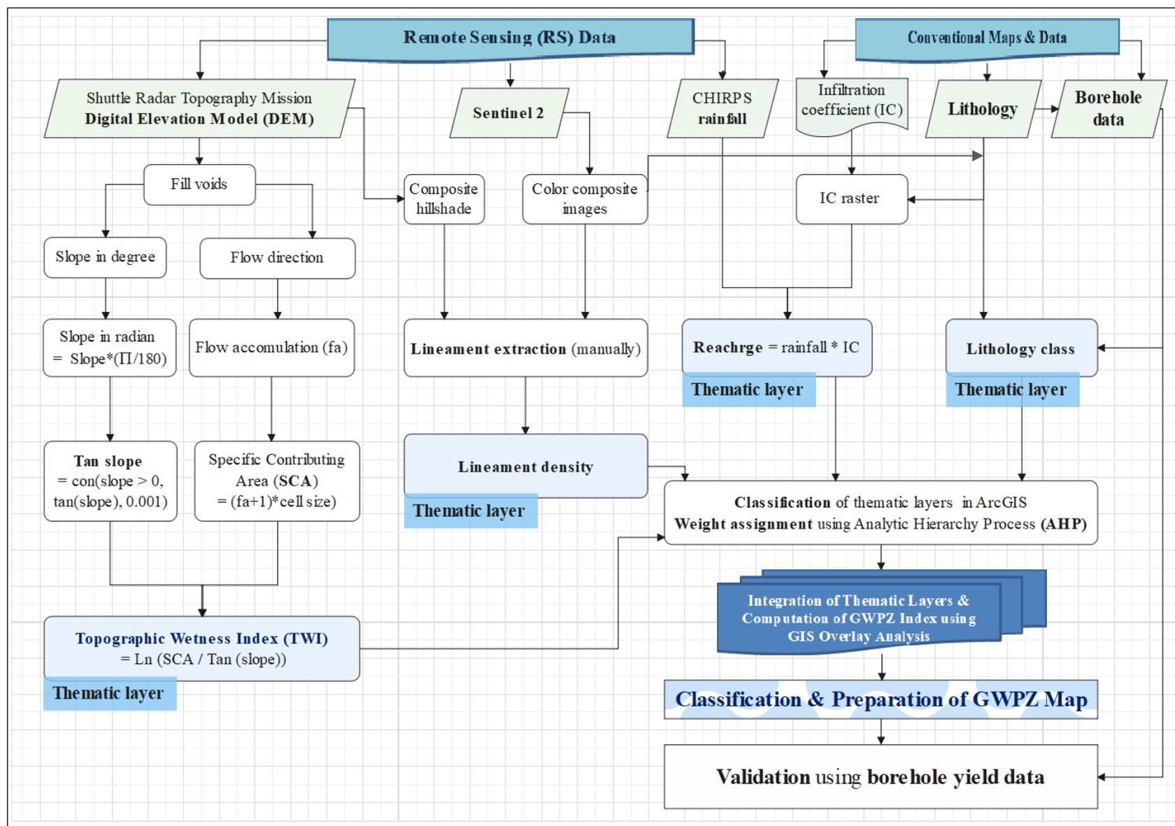
Figure 4.1. Flowchart for mapping of groundwater potential zones using using GIS Overlay technique.
